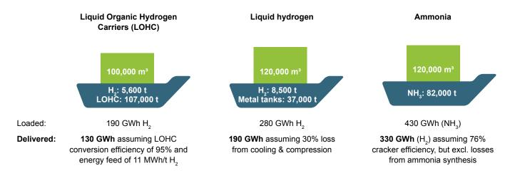
Note: all numbers rounded. Weight, volume or energy delivered does not consider energy consumed as shipping fuel \* Ship and tank dimensions based on a large tanker vessel with a maximum cargo carrying capacity of 120,324 m<sup>3</sup> or 107,115 Deadweight Tons. In reality, the vessel type may differ depending on the cargo transported.
