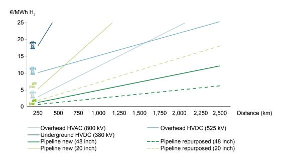
Figure 4.6 Cost comparison of hydrogen transport routes: electricity and pipelines
