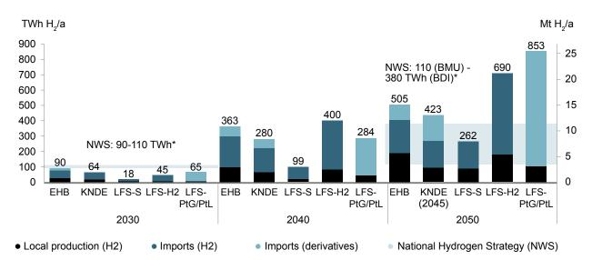
Projections: NWS: National Hydrogen Strategy, EHB: European Hydrogen Backbone, KNDE: Climate-Neutral Germany 2045, LFS: Langfristszenarien (-S: electricity scenario, -H2: hydrogen scenario, -PtG/PtL: power-to-liquid/power-to-gas scenario). \* Includes both hydrogen and PtG/PtL demand.
