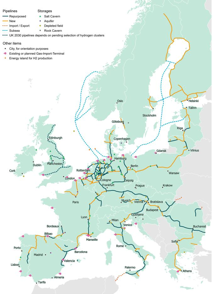
In 2030, the European hydrogen infrastructure could have a total length of around 28,000 km (see Figure 4.2). Between 2030 and 2040, the European Hydrogen Backbone will continue to grow, covering more regions and developing new interconnections across Member States. By 2040, the proposed backbone can have a total length of almost 53,000 kilometres<sup>1</sup>, consisting of approximately 60% repurposed existing infrastructure and 40% of new hydrogen pipelines (see Figure 4.3).
