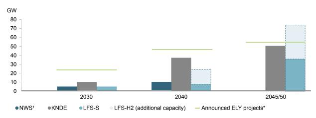
Projections shown: NWS: National Hydrogen Strategy, KNDE: Klimaneutrales Deutschland 2045, LFS: Langfristszenarien (-S: electricity scenario, -H2: hydrogen scenario). Areas with dashed outlines show theoretically needed electrolysis (ELY) capacity assuming an electrolysis efficiency of 70% and 3,500 full
